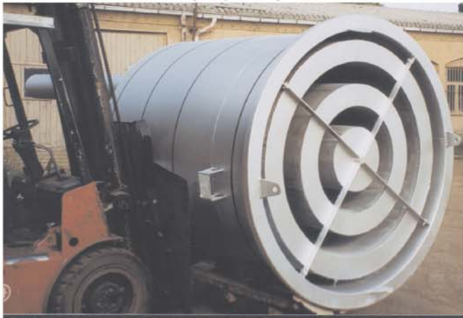
60 t/hr blow off silencer during lorry loading
