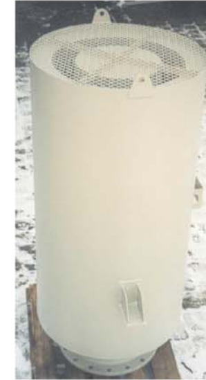
Air Blower Bypassilencer 20.000Nm 3 /hr
