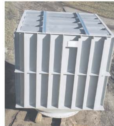
Silencer upstream ventilator, designed for +/- 9.500 Pa. Stiffeners acc. to stacical analysis
